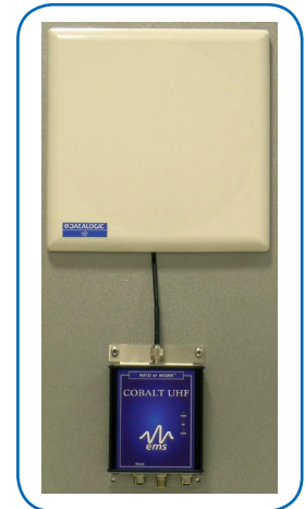
Antenna with Cobalt UHF Controller
